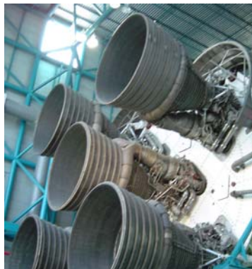
Another view of the huge Stage One engines on Saturn V which generated 7.5 million pounds of thrust at liftoff.
